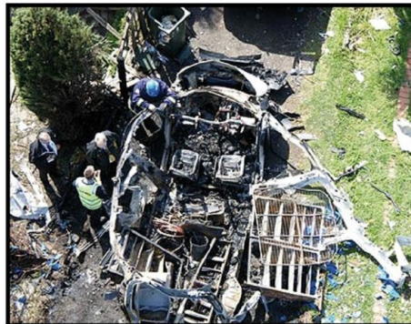
AFTERMATH OF A FLAMMABLE GAS EXPLOSION INSIDE A VEHICLE
