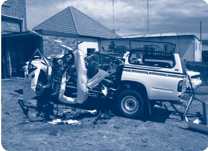
Above: Aftermath of an explosion caused by a buildup of flammable gas in a vehicle.
